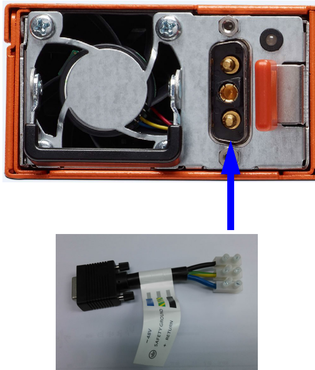
Figure 4-4: Connecting DC Power Supply Module
