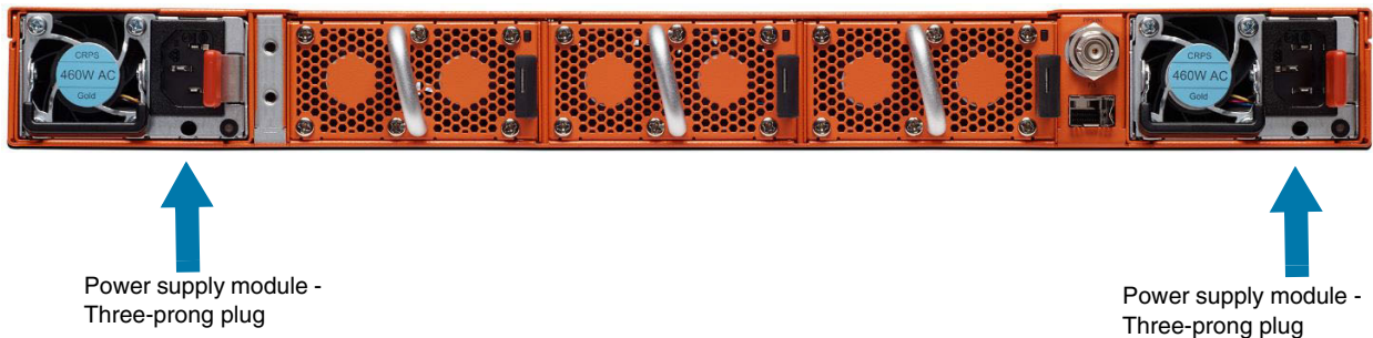
Figure 4-2: Connecting AC Power (GigaVUE-HC1)
